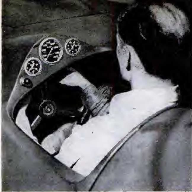
Instruments are few on the tiny dashboard. At 275 miles an hour, the driver can't be looking at dials
